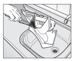
■ Clean the fabric conditioner channel using a brush and hot water.
